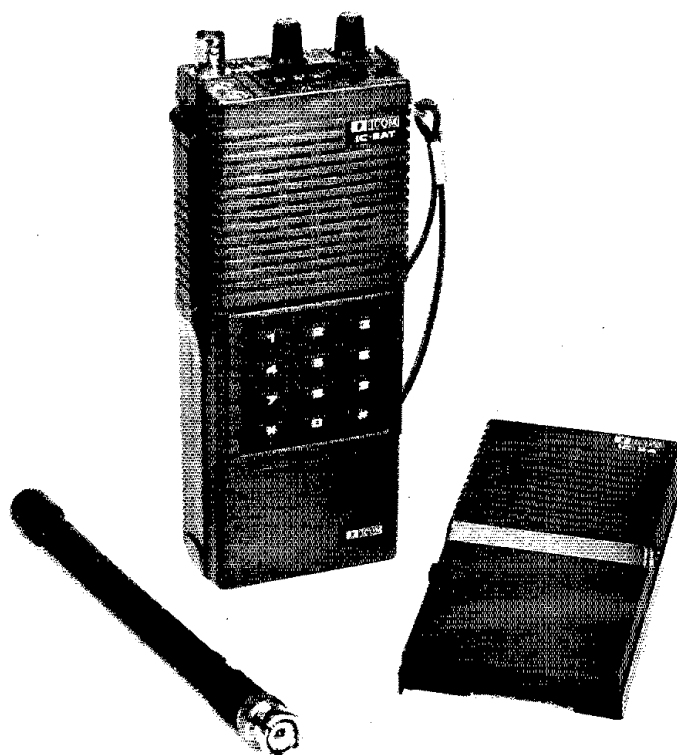
Fig. 1 — The IC-2AT. A BNC antenna connector permits rapid and positive antenna connections to be made. The flexible antenna is a part of the standard package. To the right of the transceiver is the original case front. Conversion from the IC-2A to IC-2AT is discussed in the text.
